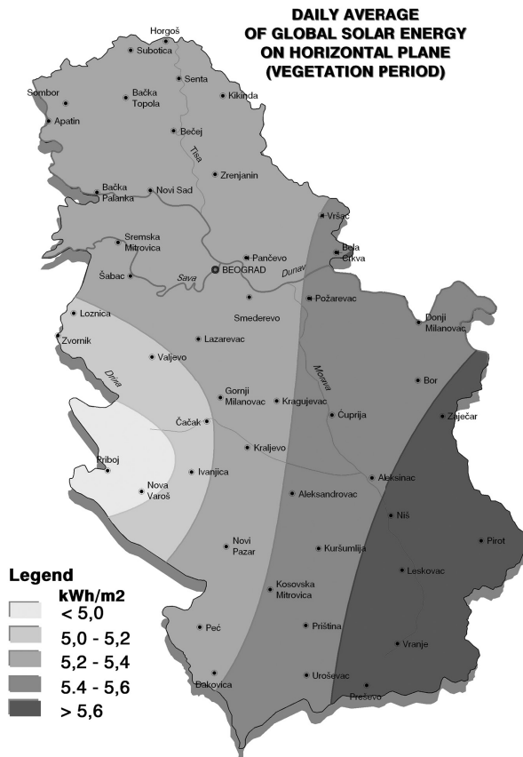
FIGURE 5.2. – Map of the daily average of global solar energy on the horizontal plane in Serbia for vegetation period (April – September), (Source: Gburcik V. et al., 2008)
